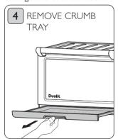
To remove crumbs, slide out the crumb tray and discard crumbs. Wipe clean and replace.
